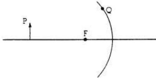
1. An object 6 centimeters high is placed 30 centimeters from a concave mirror of focal length 10 centimeters as shown above.
