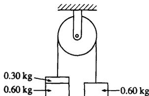
6. Two 0.60-kilogram objects are connected by a thread that passes over a light, frictionless pulley, as shown above. The objects are initially held at rest. If a third object with a mass of 0.30 kilogram is added on top of one of the 0.60-kilogram objects as shown and the objects are released, the magnitude of the acceleration of the 0.30-kilogram object is most nearly
