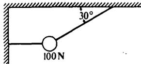
8. A 100-newton weight is suspended by two cords as shown in the figure above. The tension in the slanted cord is
